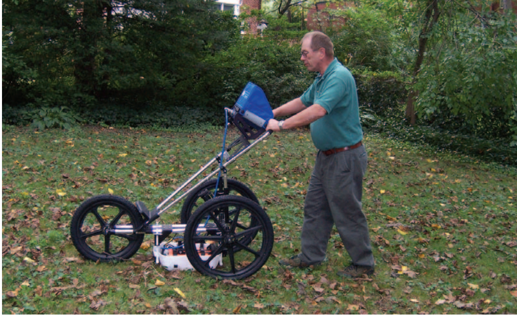
TreeRadar also scans below ground to examine the number, location, length and density of tree roots, and can also detect underground utilities or signs of past trenching that can weaken the tree from below.
